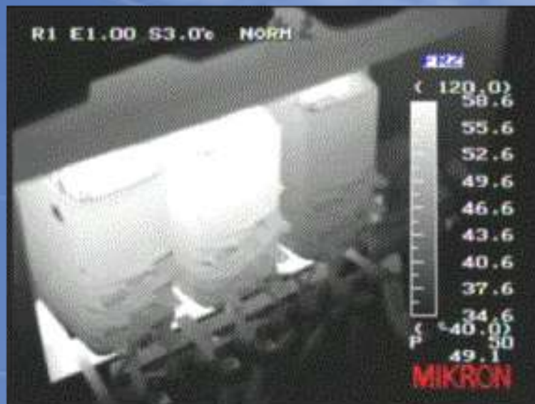
Above thermal and daylight images show uneven heating in the windings of a three phase step-down transformer, most likely due to harmonics.
